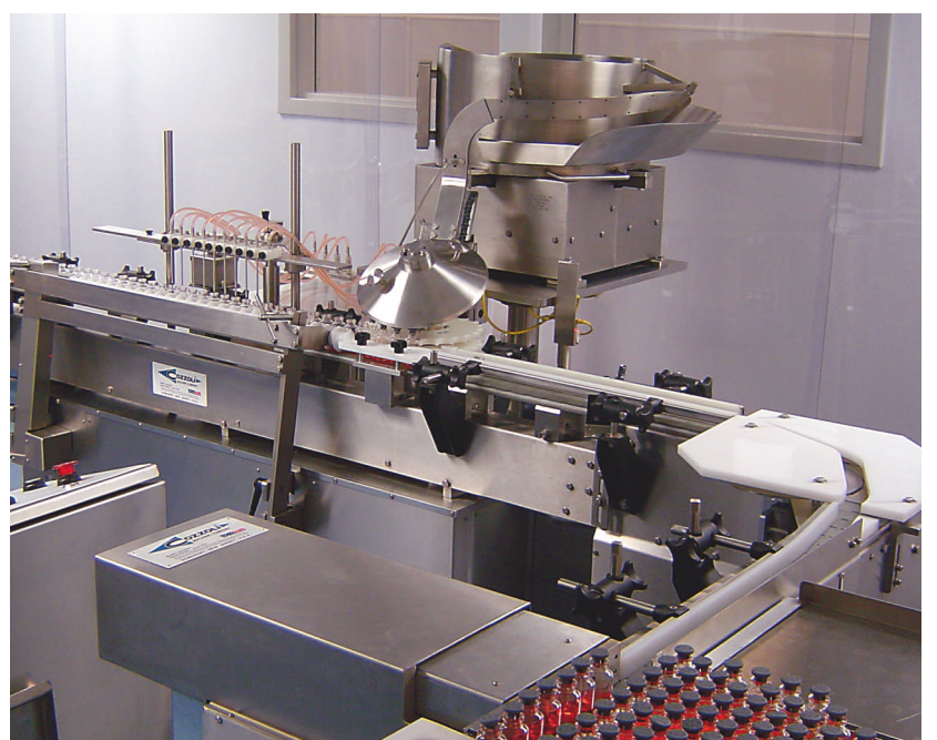
After filling, vials enter the stopperer, which inserts stoppers into the vials. The vials are then conveyed around the corner to the dual-tray loader.
