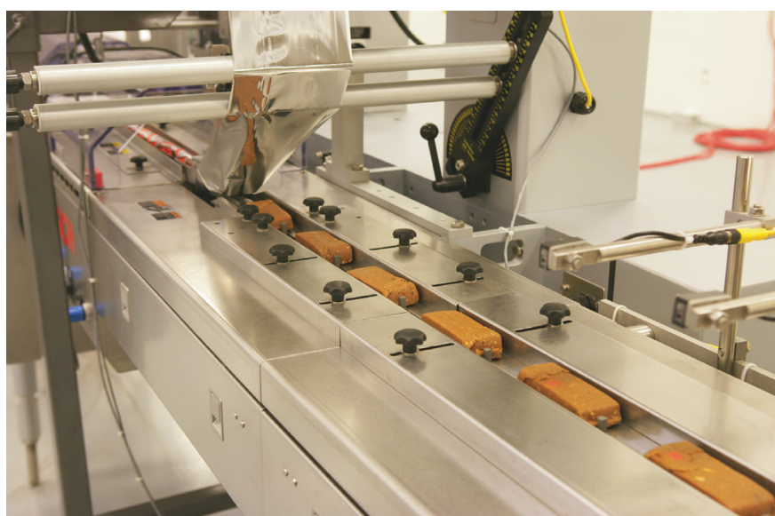
The wrapper's servo-driven infeed conveyor interfaces with the robotic placer to provide variable speed based on product flow as well as proper placement with incredible accuracy.
