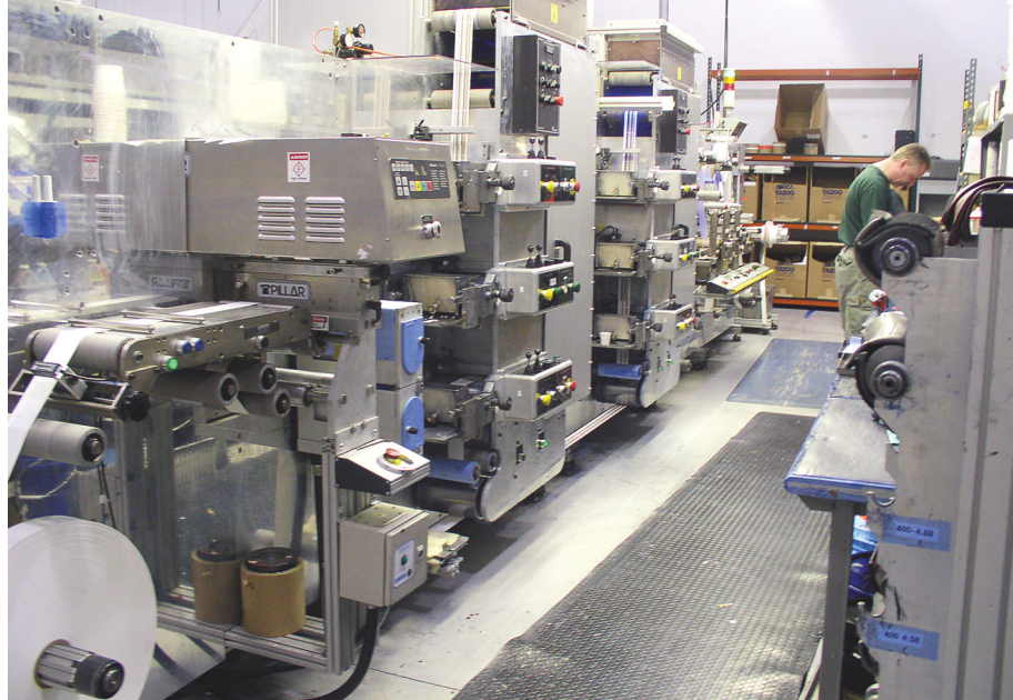
A six-color flexo press stationed in the Estée Lauder workcell is used to print its p-s labels.
