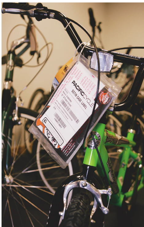
An RFID tag is embedded into a shipping label, which is hung on the bike's handle bars. The tags are also applied to cases and pallets.
