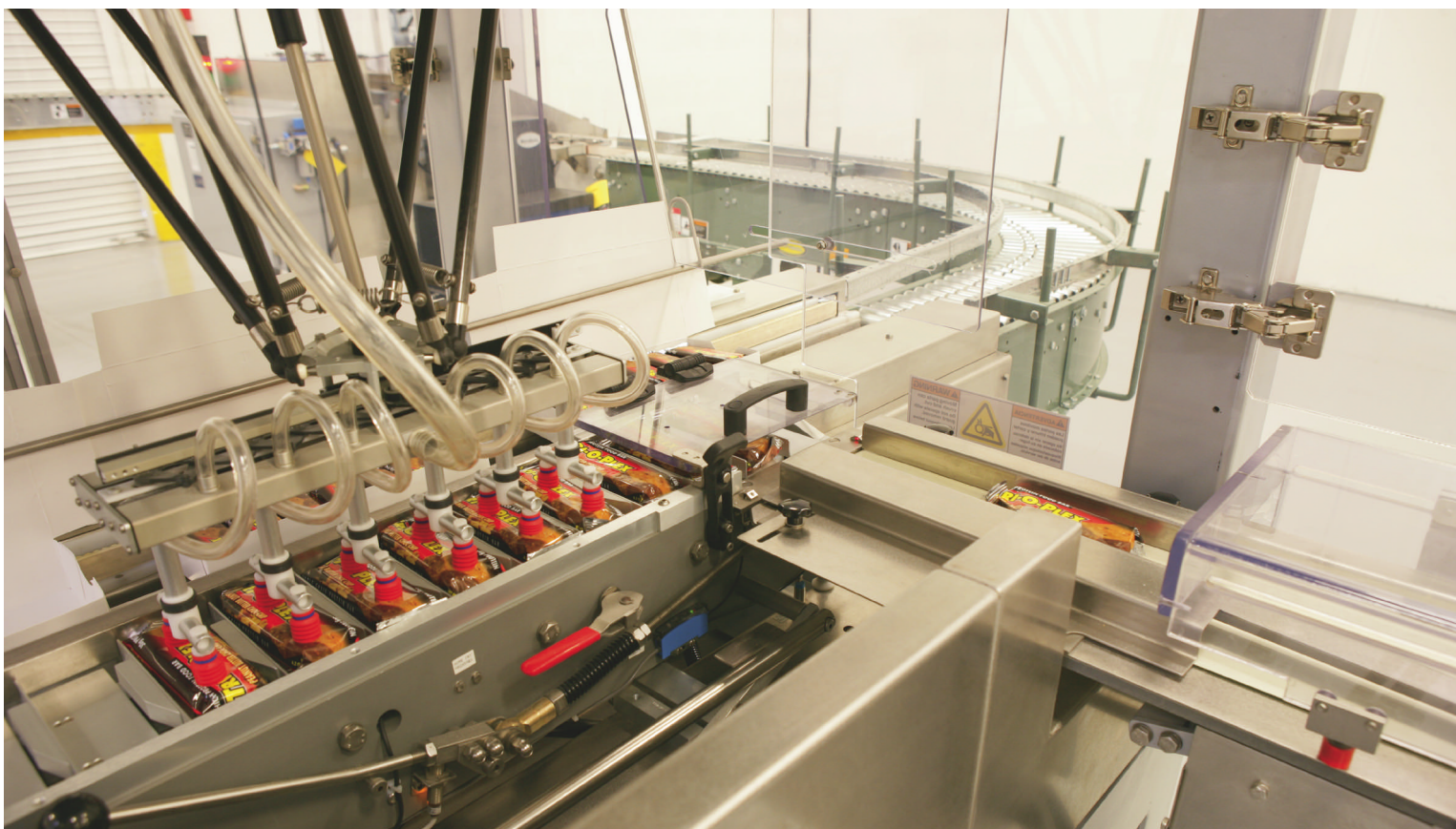
A top loader uses vacuum-cup end effectors to pick up wrapped bars and place them in rows and layers in cartons. Advanced tracking software is capable of picking the product out of a moving collation chain and top-loading the moving carton at speeds up to 400 bars/min.
