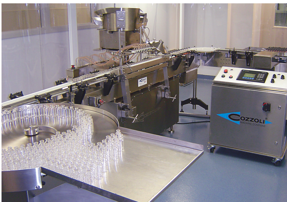
The vial line starts with a rotary unscrambling table from which vials are single-filed to the in-line filler, which fills 10 vials at a time. Product is dispensed by positive-displacement piston pumps.
