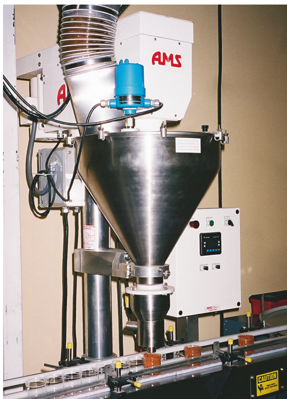
Auger fillers on both the bottling line, above, and the vertical form/fill/seal machine are equipped with programmable logic controllers and operator panel that store operating parameters for numerous products.
