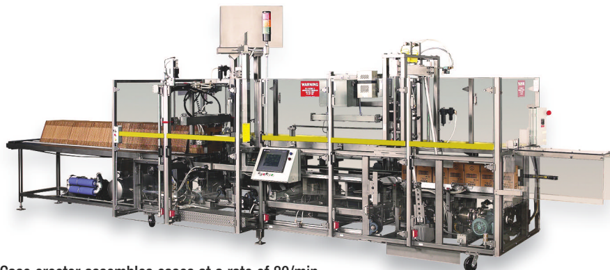
Case erector assembles cases at a rate of 80/min.
